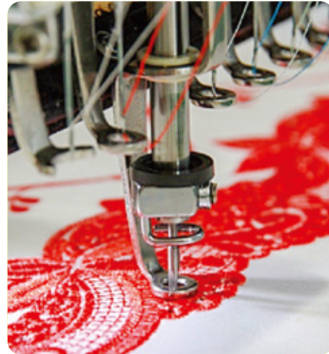
Boring Needle This specifically designed needle creates intricate embroidery by piercing the fabric, cutting it into various shapes, and leaving holes in the item.
